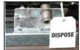
The LOV bulk oil manifold is shown above and right. The fill line is on the left. The dispose is on the right next to the Hirschmann plug.
