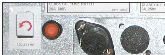
The orange JIB reset button (shown above on a McDonald's LOV fryer) is pressed to reset the system and pressed and held to refill the JIB from the bulk oil system.
