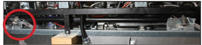
The LOV bulk oil manifold is shown above and right. The fill line is on the left. The dispose is on the right next to the Hirschmann plug.
