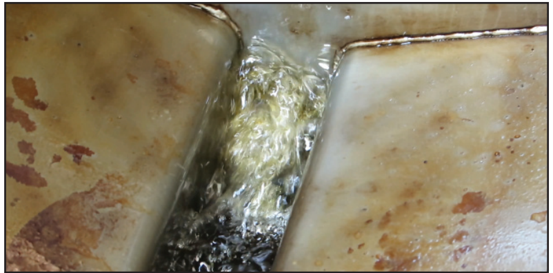
Failure to refill the frypot after a filter cycle causes heating failures. The problem is often related to cleaning the frypot, filter system.
