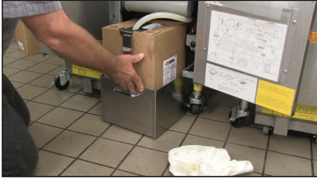
A JIB (Jug in a Box) is shown being placed in a fryer cabinet.
